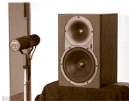
Typical microphone and equalized speaker placement used in impedance tests.
