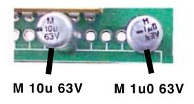
Make sure to read the capacitor correctly.
